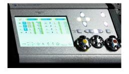
SM10 remote<sup>touch</sup> includes a unique feature which allows locking each of the manipulators individually to the microscope movement without using a PC connection! Everything is calculated in real time.
