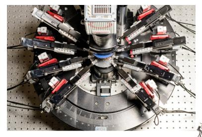
The new design of our LNprism, which manufactured in one piece! offers a better prism stability. Together with double of the thickness, this new version of our prism offers the ability to exchange electrodes with zero vibrations.
